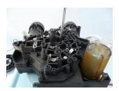
11) Replace the top plate positioning it over the flappers and pressing it down and the secure each screw. Do this randomly and it is a good idea to reverse turn each screw so that the screw drops into the existing thread and tighten. Do not over-tighten
