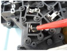
12) Re-engage each of the springs into the hole in the flapper valve. Ensure these are in and secure. You can test by pushing each of the flapper valves towards the spring and ensure the spring closes the valve after tension is released. As in the picture below
