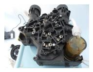
6) Undo the Connection of the Brine tube to the air-check valve and just push to one side leaving full access to the top plate and springs
