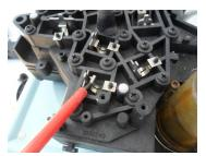
7) With a small screwdriver un-hook each of the stainless steel springs. Note some springs will be doubled. i.e. One on top of the other. Do not attempt to remove the springs off their seating pin
