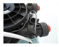
18) Re-secure the Brine Tube to the air-check valve
