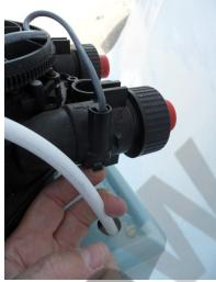
2) Unclip the Turbine Sensor from the rear port. Gently push the clip and it will pull out easily
