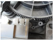
16) Now replace the Control Panel but ensure that the contact switch arm at the back is held in so that it is free of the Main cog and this allows the control panel to clip into place. Be VERY CAREFUL NOT TO BREAK THE CONTACT ARM
