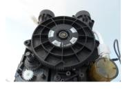
5) Now proceed to remove the motor by removing the two silver covered screws. The Motor and Control Panel can be put to one side leaving clear access to the top plate
