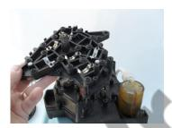
9) Remove the top plate and springs and now you have access to the flapper valves
