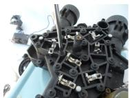
8) Now un-do all of the top plate securing screws. Do not remove the screws as it is best to ensure that the screws go back into the same hole. Not essential but advised so the threads in the plastic moulding beneath are identicle
